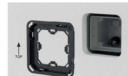
5a Insert the box into the hole at a depth from 9 to MAX 20 mm compared to the flush wall
